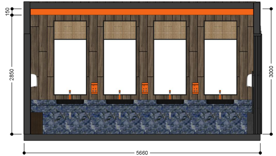
ELEVATION A PUBLIC TOILET scale 1:35
