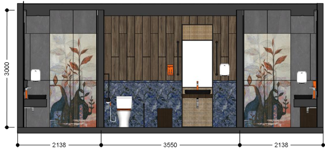
ELEVATION B PUBLIC TOILET scale 1:35
